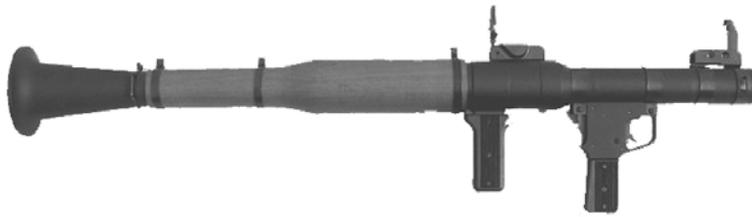
RPG 7 launcher (bore diameter 1.57 inches)
